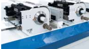
Flexo unit for printing, varnishing and Coldfoil or linerless laminating.
